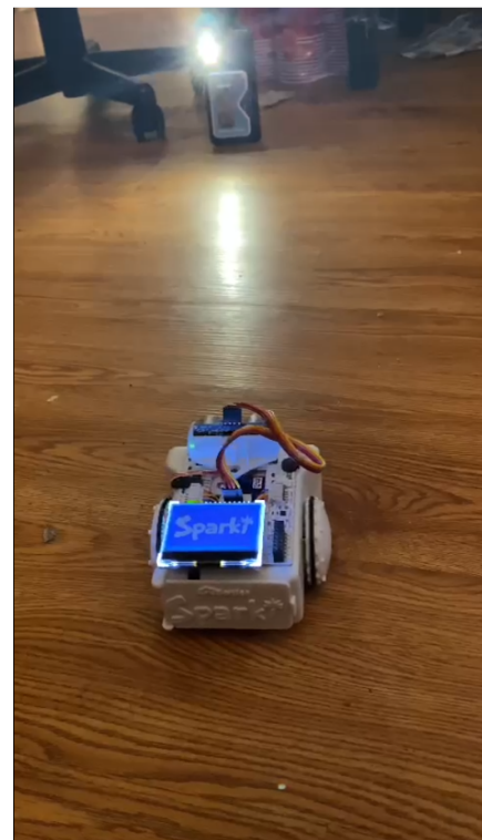
Figure 7. Sparki following light
