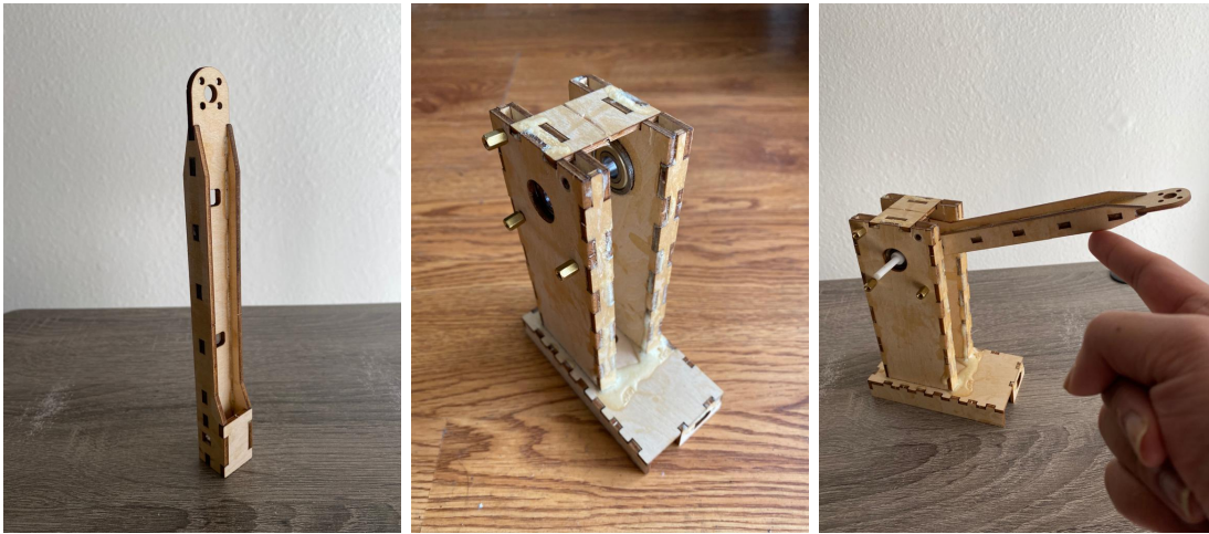
Figure 4: Arm assembled and a cut made on the top part
